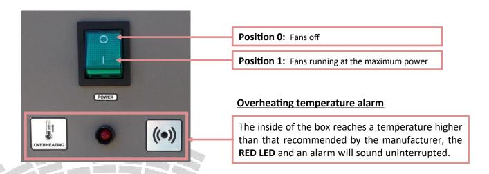
**NOTE:** If this happens, simply open the cover to vent the gas generator. Later, check that the fans work correctly.
